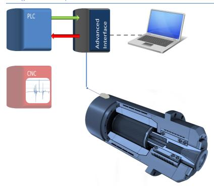
With the advanced interface up to 3 relay alarms can be sent to PLC. One of the alarms is linked to collision events while the other two are linked to RMS vibration velocity thresholds exceeded during working process.
